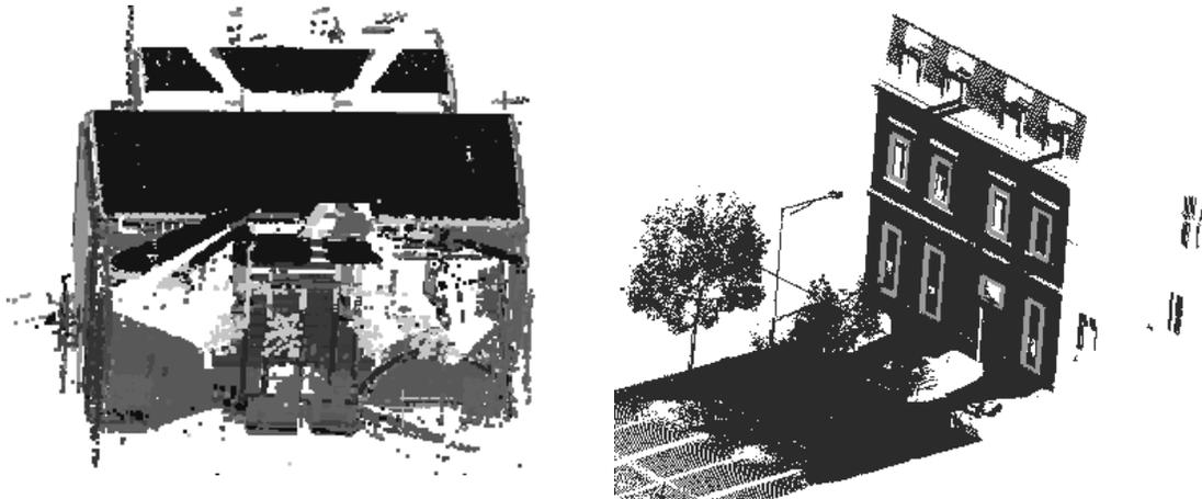
Fig. 3: Feature extraction in LiDAR scans. Left: planar regions detected in an indoor scan. Right: Openings detected in an outdoor scan.
